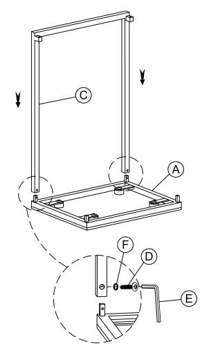
Step 2: Do not fully tighten the bolts
